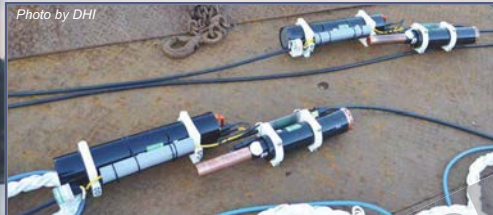
WQM-Dredges with Inductive Modem Modules & battery packs
