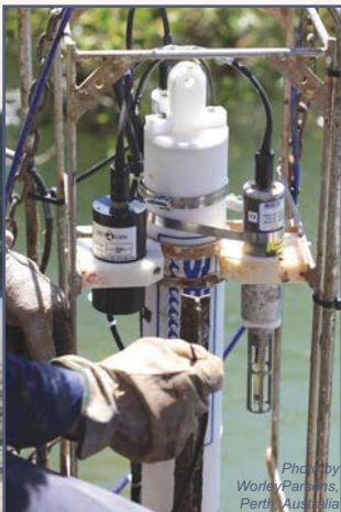
SBE 16plus V2 SeaCAT CTD with SBE 18 pH & WET Labs ECO-NTU with Bio-wiper™
